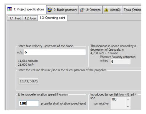
• Select the blade geometry / dimensions blade tab to enter the radius blade tip and blade root radius(diameter of the propeller, and the hub): By varying the swept section, we will control the axial velocity for the given flow 12 m/sec.
