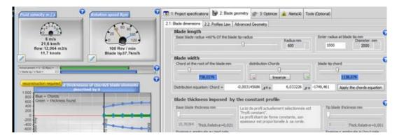
Changing the speed or blade length, leads, of course, the change in flow. We have chosen the values of velocity and length giving us the **flow rate imposed 12 m3/sec.**.
