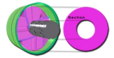
• Velocity axiale(m/sec) = flow (m3/sec) / swept section (m2)
