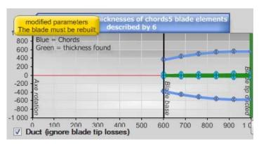
Ticking the option Duct relaunch calculation of the propeller..
